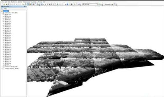
Figure 2. An example of Digital Surface Model (DSM) concerning all the tiles of the municipality of Portici in 2D, above, and 3D, below. Elaboration by D. Pavia & C. Pesaresi
