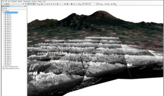
Figure 3. An example of Digital Surface Model (DSM) concerning all the tiles of the municipality of Portici with the overlay of a Digital Terrain Model (DTM) which shows the morphology of the Somma-Vesuvius complex, above, or with a specific overlay of a satellite image ("Sentinel 2") which provide further elements in terms of visualization, below. Elaboration by D. Pavia & C. Pesaresi.
