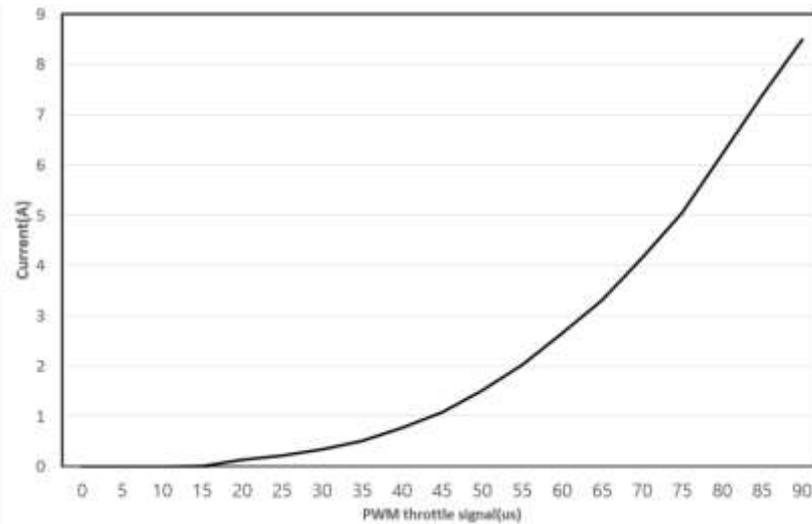
Fig. 6. Current consumption measurement result according to PWM throttle change
