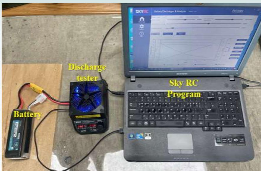
**Fig. 7.** System of the discharge test
