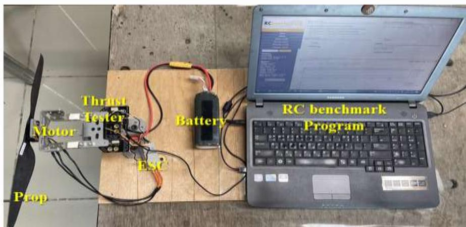
**Fig. 4.** System of the thrust test
