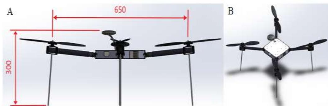
**Fig. 1.** 3D design of the 650 mm unmanned drone for greenhouse: A, Size of the 650 mm unmanned drone; B, Isometric of the 650 mm unmanned drone
