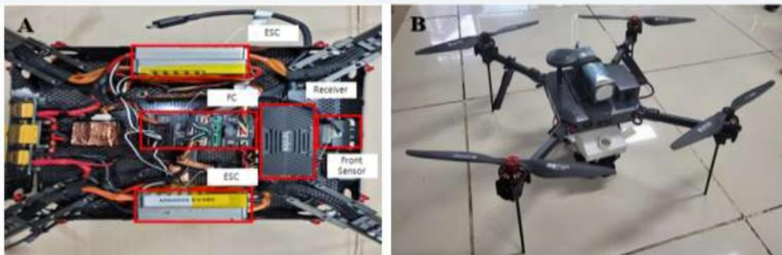
**Fig. 3.** The developed unmanned drone for greenhouse: A, Main parts inside the drone; B, Fabricated of the drone
